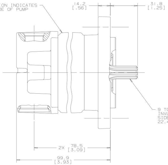
9 TOOTH 16/32 DP 30° INVLT FLAT ROOT CLASS I SIDE FIT SPLINE SAE J4986b 22.4 [.88] MIN FULL SPLINE
