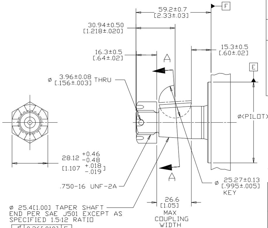
Ø 25.4[1.00] TAPER SHAFT END PER SAE J501 EXCEPT AS SPECIFIED 1.5:12 RATIO
